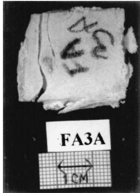
Figure 19 Fracture of reinforced syntactic foam specimen tested under compression in orientation 1.
