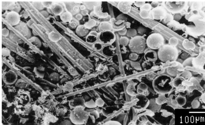
Figure 21 Undamaged microballoons in reinforced syntactic foam specimen tested in orientation 1.
