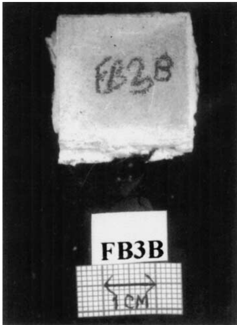
Figure 20 Fracture of reinforced syntactic foam specimen tested under compression in orientation 2.
